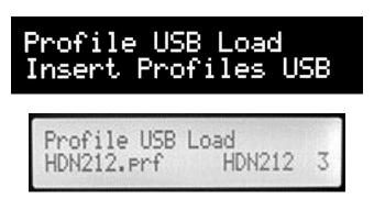
➡ Once loaded into one of the twelve B|AMP's Profile memory slots, the new speaker profile can be loaded into the B|AMP's Profile EQ filters by cycling back to the Profile Select menu and turning the Bass/Filters knob until the desired profile name is indicated on the OLED display.
